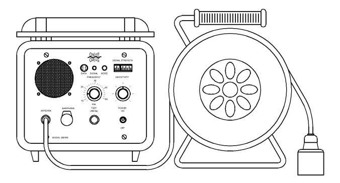
The 2001RS Pinger Receiver is a portable, battery powered, acoustic receiver, tuneable to all frequencies between 8 kHz and 50 kHz which can be used for tracking and locating underwater acoustic transmitters. The receiver has loudspeaker and headphone audio outputs, an easy to interpret signal meter, simple frequency and sensitivity controls and self-test / battery test functions. The 2001RS is used with the OEL Standard Hydrophone when deployed.
