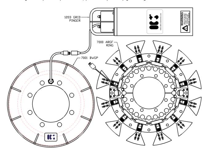
The current system can be manufactured to specific project specifications and supplied with a 600, 800 or 1200 sized GRID<sup>®</sup> Pinger. These are based on Online's proven 600, 800 and 1200 series acoustic pinger designs. The 7000 ARGF Ring is typically suitable for 10'' pipelines or larger.
