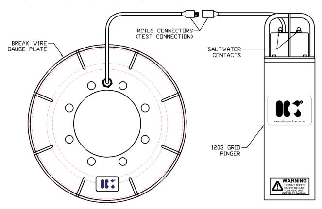
If the connection between the BWGP and GRID® Pinger is broken while the system is activated, the GRID® Pinger will respond as if the gauge plate has been damaged. This simple behaviour can be used to test the system. Note: If testing the GRID® System in air, the acoustic hydrophone should be placed within 10cm of the transducer head on the GRID® Pinger. If using a GRID® Pinger with frequency below  $\sim 15 \, \text{kHz}$ , the acoustic transmissions should be audible without using a receiver.
