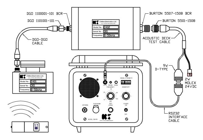
Prior to installation with the ROV and ROV umbilical, ensure that the system deck test has been completed. This will confirm that the system components are functional prior to installation on the ROV and familiarize the user with the equipment, installation, and operation. In this test the ACOUSTIC DECK TEST CABLE takes the place of the ROV and ROV umbilical.
