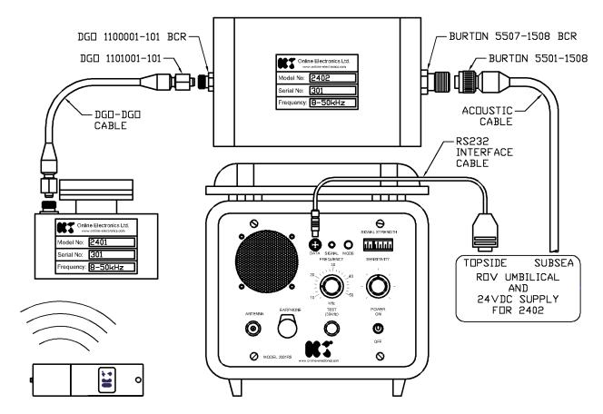
Prior to installation with the ROV and ROV umbilical, ensure that section 4.1 ROV SYSTEM DECK TEST has been completed. This will confirm that the system components are functional prior to installation on the ROV and familiarize the user with the equipment, installation, and operation. Note that the diagram above shows the standard connector (BURTON 5507-1508 BCR) on the 2402, alternative connectors such as SEANET may be fitted if requested at time of order.
