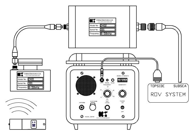
The 2001RS Pinger Receiver is a portable, battery powered, acoustic receiver, tuneable to all frequencies between 8 kHz and 50 kHz which can be used for tracking and locating underwater acoustic transmitters. The receiver has loudspeaker and headphone audio outputs, an easy to interpret signal strength meter, simple frequency and sensitivity controls, and self-test / battery test functions. The 2001RS is used with a 2402 acoustic pod and 2401 ROV hydrophone when deployment via ROV is required.
