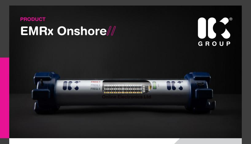
THE ONLINE ELECTRONICS EMRX ONSHORE RECEIVER IS A ROBUST, STATE OF THE ART, MULTI-FREQUENCY, ELECTROMAGNETIC (EM) RECEIVER USED FOR LOCATING LOST OR STALLED PIGS AND TRACKING PIGS FITTED WITH ANY EM PIG TRANSMITTERS. IT CAN ALSO BE USED TO CONFIRM A PIG HAS LEFT OR ARRIVED AT A PARTICULAR LOCATION AND FOR GENERAL MONITORING OF PIG MOVEMENTS.
