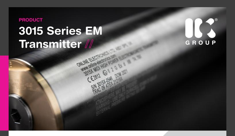
THE 3015 TRANSMITTER IS AN ATEX RATED ELECTROMAGNETIC TRANSMITTER THAT CAN BE USED FOR PIG TRACKING AND LOCATING FUNCTIONS, INTENDED FOR USE IN PIPELINE DIAMETERS ABOVE 10". THE TRANSMITTERS OPERATE EFFECTIVELY IN EVERY TYPE OF PIPELINE, I.E TOPSIDE, BURIED, GAS OR LIQUID AND IN PIPELINE BUNDLES WHERE ACOUSTIC TRANSMITTERS ARE EITHER LESS EFFECTIVE OR INEFFECTIVE.
