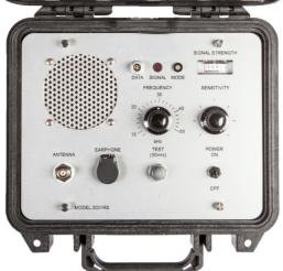
THE 2001RS PINGER RECEIVER IS A PORTABLE, BATTERY POWERED, ACOUSTIC RECEIVER, TUNEABLE TO ALL FREQUENCIES BETWEEN 8 kHz AND 50 kHz WHICH CAN BE USED FOR TRACKING AND LOCATING UNDERWATER ACOUSTIC PINGERS.
