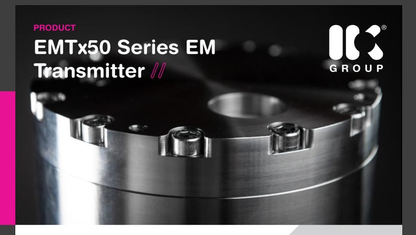
THE EMTX50 TRANSMITTER IS AN ELECTROMAGNETIC TRANSMITTER THAT CAN BE USED FOR PIG TRACKING AND LOCATING FUNCTIONS, INTENDED FOR USE IN PIPELINE DIAMETERS OF AROUND 16" AND ABOVE. THE TRANSMITTERS OPERATE EFFECTIVELY IN EVERY TYPE OF PIPELINE, I.E. TOP-SIDE, BURIED, GAS OR LIQUID AND IN PIPELINE BUNDLES WHERE ACOUSTIC TRANSMITTERS ARE EITHER LESS EFFECTIVE OR INEFFECTIVE.
