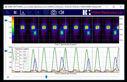
THE ONLINE ELECTRONICS EMRX WINDOWS APPLICATION CAN BE USED IN CONJUNCTION WITH ALL EMRX RECEIVERS FOR LOCATING LOST OR STALLED PIGS AND TRACKING PIGS FITTED WITH ANY ELECTROMAGNETIC (EM) PIG TRANSMITTER. IT CAN ALSO BE USED TO CONFIRM A PIG HAS LEFT OR ARRIVED AT A PARTICULAR LOCATION AND FOR GENERAL MONITORING OF PIG MOVEMENTS.
