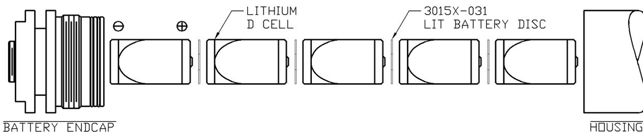
7. Once all cells are installed ensure that it is the FLAT, NEGATIVE END of the cells which you see when looking into the open end of the transmitter.
